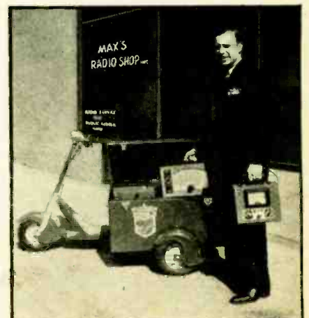
Mr. Service Man: The scooter model shown above is a 3-wheeler, having a convenient side trunk (taking the place of the usual side car in the motor cycle) in which can be carried all the necessary service instruments, tools and manuals for any service call.
